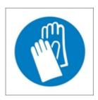
Hand protection Wear protective nitrile rubber gloves. Thickness ≥ 0.38 mm - breakthrough time >480
